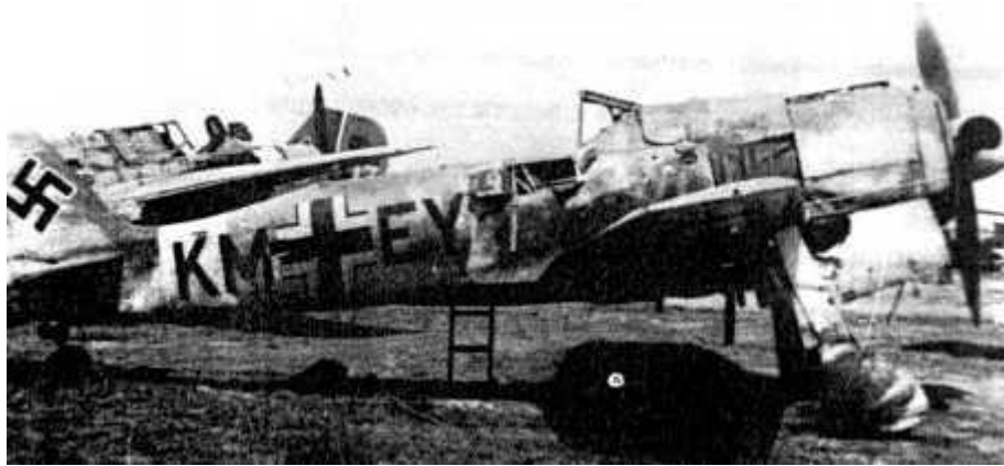
Figure 15 - Relatively few FW 190A-5s reached Tunisia before the German evacuation. This derelict carries the standard 74/75/76 factory finish with the 4 letter radio call sign KM+EY and white rear fuselage band and wingtips. Damage to the engine was probably responsible for the fouling over the wing roots and wheel covers. In the background is an Hs-129B of 8./SchG.2 with an unusual mottled scheme, possibly of 79/80, who a blue 24 letter K outlined in white. Behind this is a rather battered Ju-52/3m in 70/71/65 camouflage.
