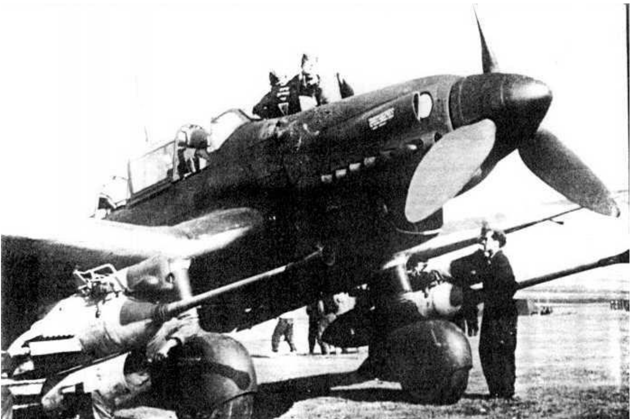
Figure 14 - Junkers Ju-87G-1 "Canonvogel" Stuka which equipped the 10(Pz) Staffel of SGs 1, 2, 3 and also part of SG.9. The underwing guns were modified 37mm AA weapons used for tank busting with all these Eastern Front units.
