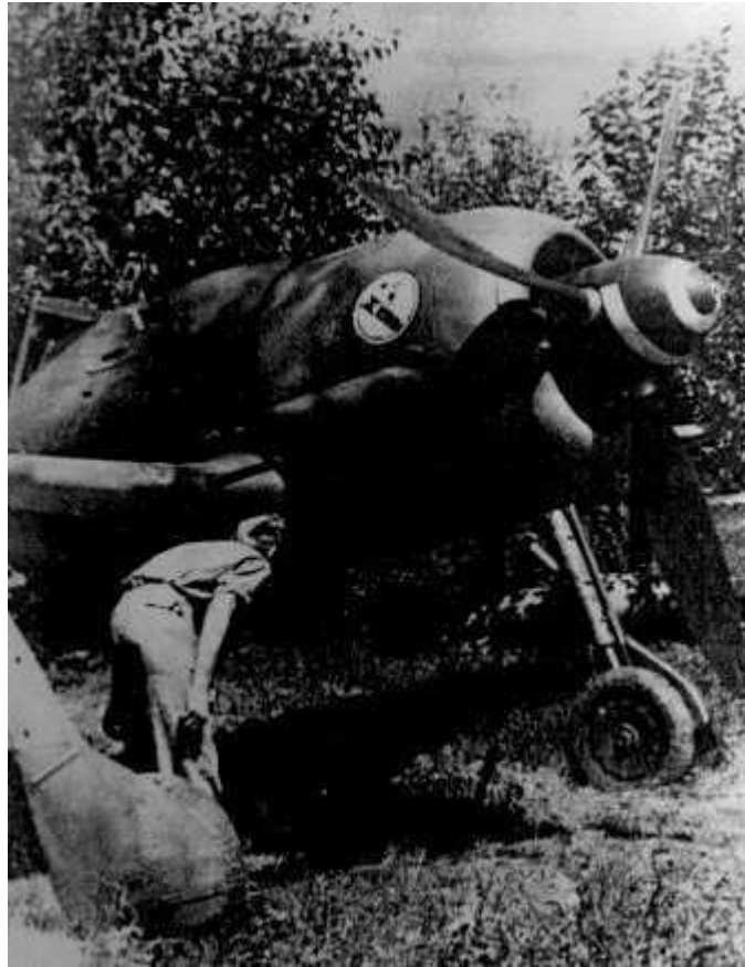
Figure 3 - FW-190/F-3 of I/SG.4 in Italy 1943. Note the unit emblem and the special spinner marking, see also the ETC501 carrier for bombs or drop tank, below.
