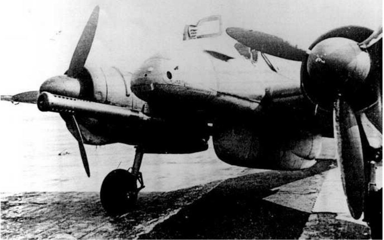
Figure 13 - A Henschel Hs-129B-2/R4 of IV/SG 9 fitted with a 75mm anti tank gun, this version was used in small numbers, as the weight of the gun made it vulnerable to enemy fighters.
