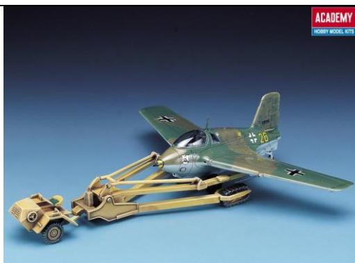
Designed for the sole objective of attacking allied bomber formation, the semi-delta wing Me163B was powered by a 3,748ld. thrust Walter rocket motor which allowed it to reach a level speed of 596mph with sufficient fuel for 8 to 10 minutes of powered flight.
