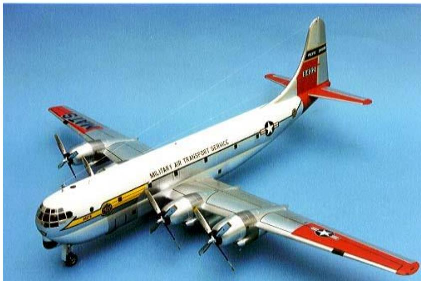
This model has been built much the same as the B-377 kit but with the addition of the COBRA resin update parts. These feature new engine cowlings with detailed engine fronts and exhausts plus late type wheels and nose steering gear, also included are the light bars which guide the receivers into station to refuel.
