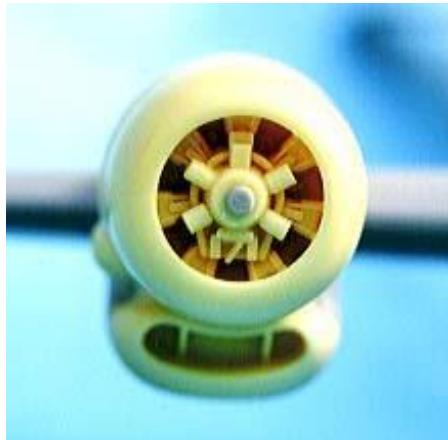
Each wing was made up as a separate item with the nacelles located and cleaned up then the pour blocks were cut off the resin engines and a final sanding cleaned up the surface. The prop mounting shafts (parts M17) won't fit now so I drilled a hole in each engine to take the shaft and cemented it in place ready to take the props.
