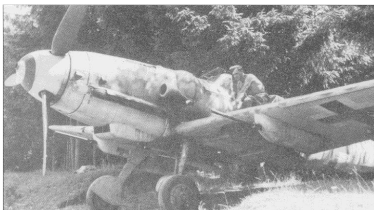
Figure 4 - A I Gruppe Me 109G-10 "Kannonboot" with underwing cannons in streamlined gondolas, designated G-10/R6, in summer 1944.
