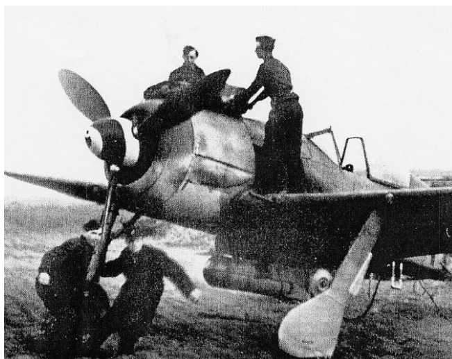
Picture 8 - FW 190A-8 of II/JG6 in Jan/Feb 1945, note container under fuselage rack, spiral spinner, lightly mottled fuselage and later war outline crosses.
