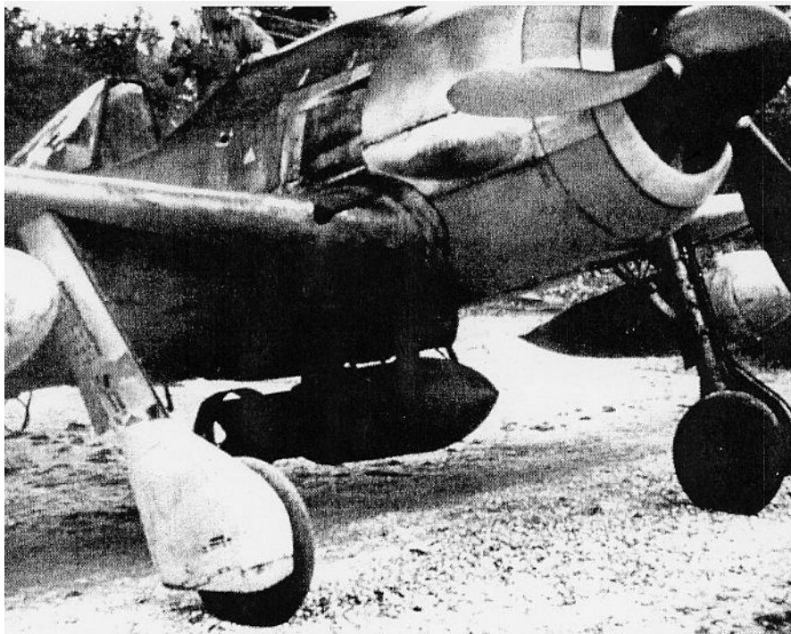
Picture 4 - FW 190a-8 of I/JG6. Note light mottle finish, halved spinner of earlier days instead of spiral. Also the SB500 bomb and 2 underwing drop tanks suggest use on the Eastern Front in Jan/Feb 1945.
