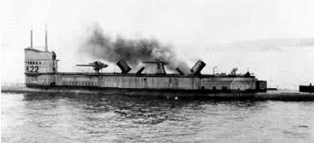
On average it took five minutes to shut off the boilers, retract the funnels, close the ventilators and hatches, evacuate the boiler room and fill the ballast tanks. Now think about trying to do all this while the enemy is blasting shells and bullets at you.
